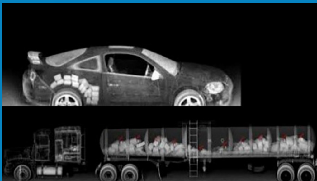
Figure 4. Images showing Cargo X-ray scanning at Customs checks with visible contraband.
